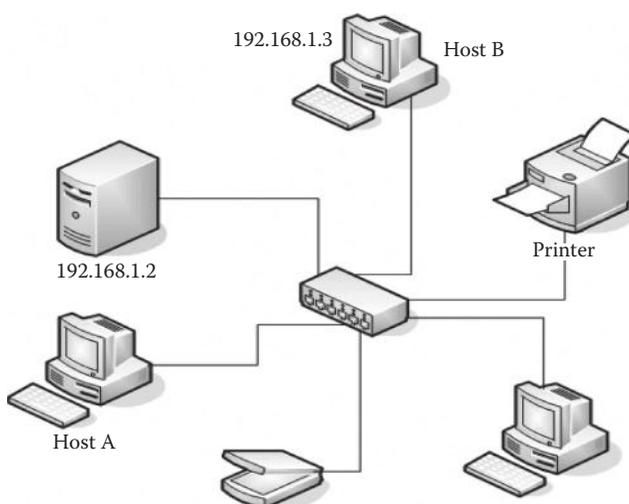
So let's imagine the scenario shown in the image, where on a switch-based network, "Host A" with an IP 192.168.1.2 would like to communicate with "Host B" with an IP 192.168.1.3. In order to communicate on a local area, Host A would need to have the MAC address of Host B.
