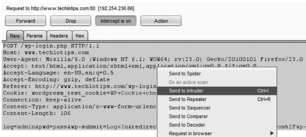
*Step 3*—Burp would automatically highlight the input fields that you can try to run your attack against; however, we are interested only in the password field with the parameter (pwd). So we will click on the “Clear” button at the right to clear all the inputs and click the “Add” button twice.
