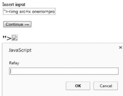
A real-world example of stored XSS that I recently came across existed in a small app created by backbonejs called “TODOS,” an application allowed users to input things to do for the day. The user input was then inserted in the local storage, and when it was reflected back, which it resulted in an XSS.
