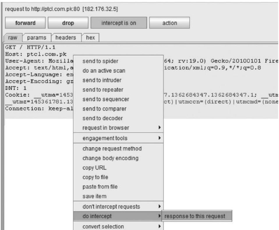
*Step 8*—Next, click on the “Forward” button to forward the http request to the server. In a few seconds, we will receive an http response, revealing the http server and its version. In this case, it is Microsoft’s IIS 7.5.
