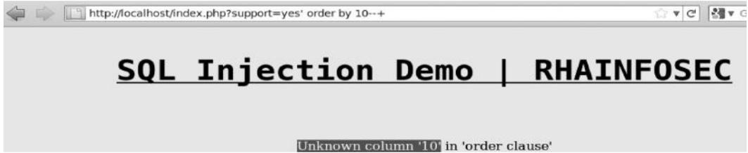
When executing this command, we get an error pointing that column number 10 does not exist. This way we know that the number of columns is less than 10. We would continue testing this way:
