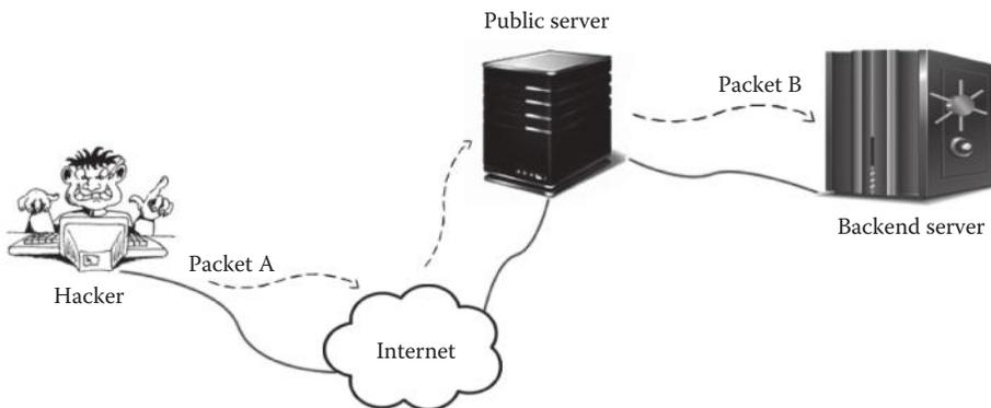
This diagram demonstrates how an SSRF vulnerability works. An attacker sends a specially crafted “Packet A” to the Internet-facing webserver and that webserver then sends “packet B” on behalf of the attacker to the back end server running on the internal network. In this way, an attacker could sometimes bypass Firewall restrictions because the back end server would trust the packet coming from the webserver as it is on the same internal network as the back end server.
