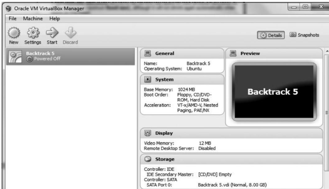
*Step 6*—So, now when the virtual hard disk has been created and other settings are selected, load the BackTrack that was downloaded onto the virtual box and click “Start”.
