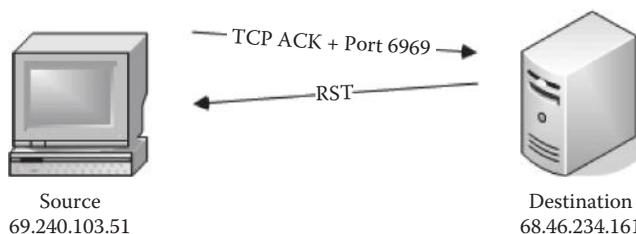
The TCP ACK scan is not used for port scanning purposes. It is commonly used to determine the firewall and ACL rules (access list) and whether the firewall is able to keep track of the connections that are being made.
