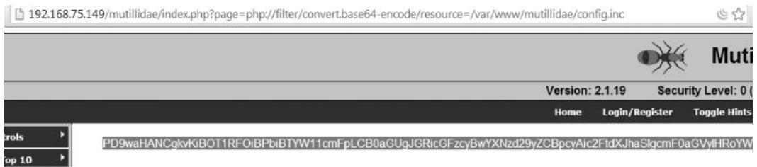
The output string returned is in the base64-encoded form; now you can use any manual online decoder to decode the base64 encoded string.
