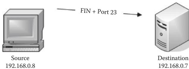
A FIN flag is used to close a currently open session. In a FIN scan the sender sends a FIN flag to the target machine: if no response comes from the target machine, it means that the port is *open*; if the target machine responds with a *RST*, it means that the port is *closed*.
