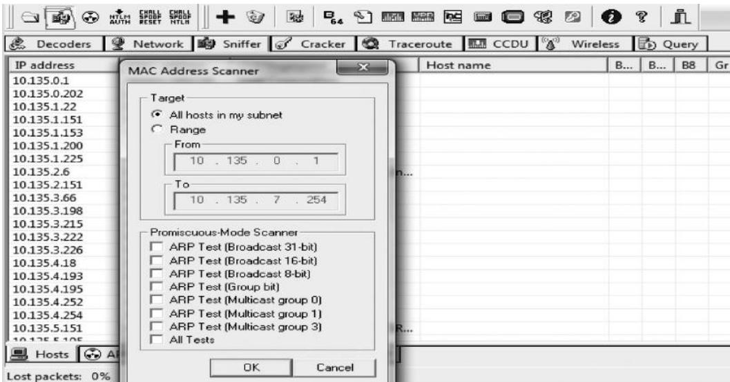
Step 3—Once you have scanned all the MAC addresses and IP addresses, it’s time to perform an ARP spoofing attack. To do that, click on the “APR” tab at the bottom and then click on the white area in the top frame. This will turn the “+” sign into blue color.
