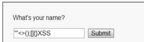
After injecting the payload from the source, we can see that no escaping is being performed on the input.
