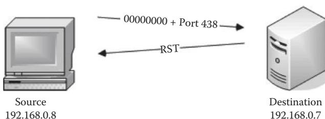
A null scan is accomplished by sending no flags/bits inside the TCP header. If no response comes, it means that the port is *open*; if a *RST* packet is received, it means that the port is *closed* or *filtered*.
