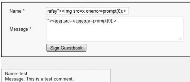
The screenshot shows a web form with two input fields: "Name \*" and "Message \*". The "Name" field contains the payload: `rafay">
