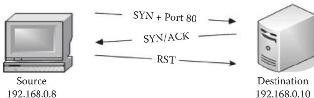
This diagram illustrates how a TCP SYN scan works:
