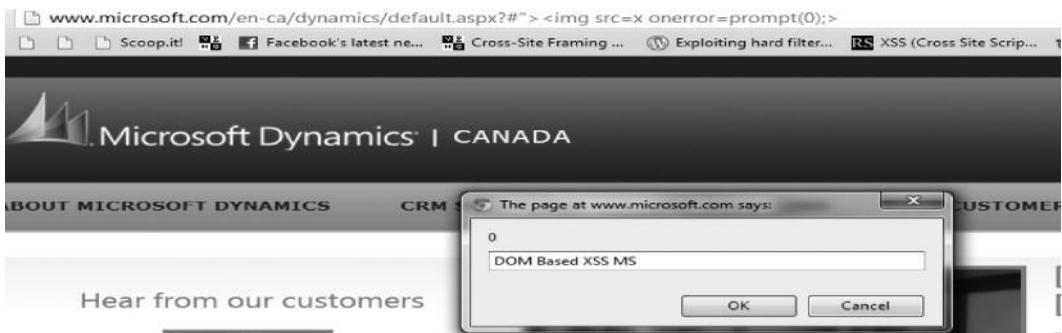
The main cause of this vulnerability was that the input passed via `location.hash` was being executed by a vulnerable sink “`Document.write`”. The Chrome js console pointed me to line 58 responsible for this vulnerability.
