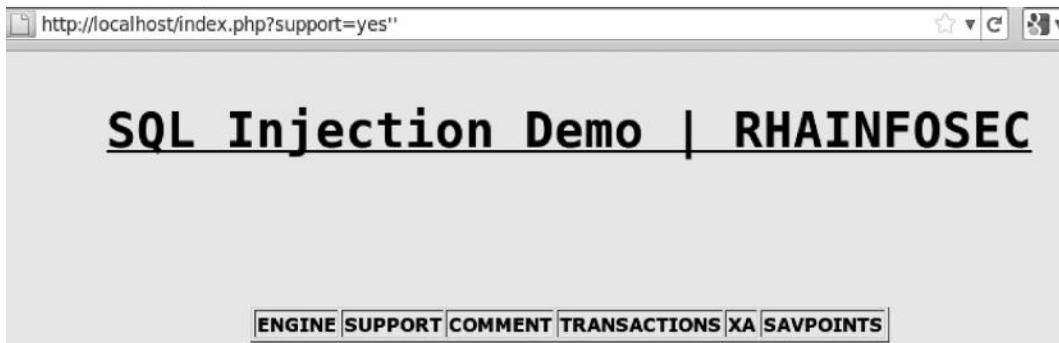
We see no error message, which means that the application is most probably vulnerable to SQL injection, because we have now defined the correct syntax.
