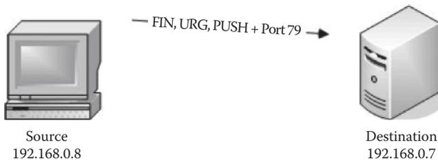
The XMAS scan sends a combination of FIN, URG, and PUSH flags to the destination. It lightens the packet just like a Christmas tree and that is why it is called an XMAS scan. It works just like the FIN and null scans. If there is *no* response, the port is *open*; if the target machine responds with a *RST* packet, the port is *closed*.
