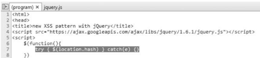
You can verify it by setting up a breakpoint on line number 7. The idea behind this is to generate an intentional error, which would get caught with Chrome js console, and hence point us to the vulnerable code.
