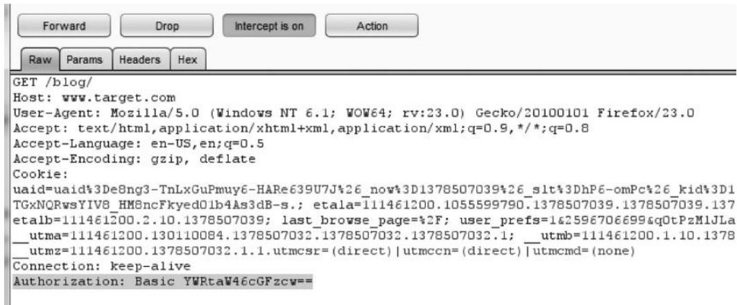
*Step 2*—Again, by default, burp intruder would pinpoint the possible positions to be brute-forced; however, we are interested in attacking only the authorization header that would be sent to the server, so we would click the “Add” button to lock the position.
