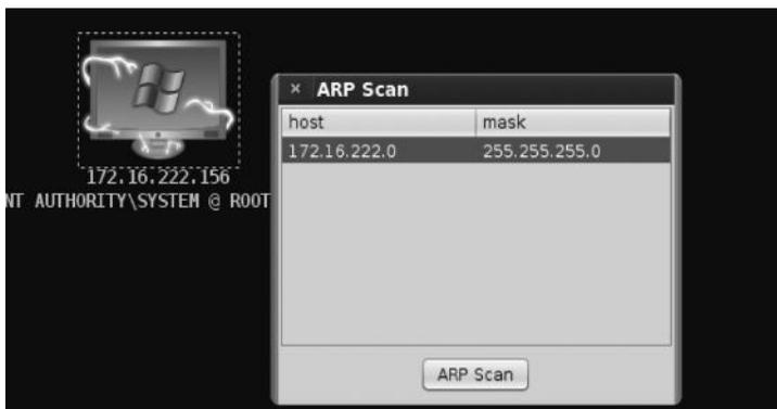
The ARP Scanner has automatically suggested that we scan the whole range 172.16.222.0–255. You can define your own ranges or choose a different subnet mask, if your target has a different one.
