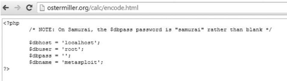
As we decoded the string, we can see the source of the configuration file that contains important information such as dbhost, dbuser, dbpass, and dbname.
