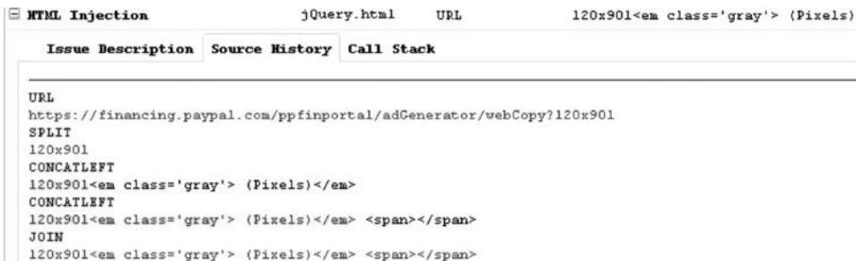
As we can see, in the first line the URL is taken from the source and a split function is called that splits everything after the question mark, then a series of concatenation is performed and finally reaches a vulnerable sink without any filtering.
