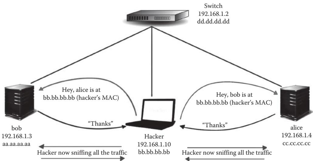
Let’s take a look at the scenario presented in this image. The hacker sniffs all the traffic using the ARP spoofing attack. We have a switch with the IP 192.168.1.2. We have two hosts, namely, “bob” with the IP 192.168.1.3 and “alice” with the IP 192.168.1.4. The “hacker” computer is also located on the network with the IP 192.168.1.10.
