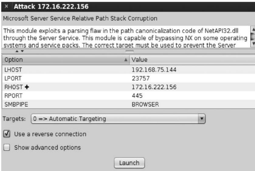
This screen is equivalent to the “show options” command in Metasploit. I have checked the “use a reverse connection” option since I want to have a reverse shell because I want the victim to connect to me. This is very helpful when the victim is behind a firewall or we cannot reach him directly.
