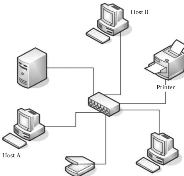
Let's assume that this topology runs on a hub-based network and that "Host A" would like to communicate with "Host B." It will forward the traffic to the hub. A hub is designed in such a way that it *broadcasts* all the traffic, meaning that it will forward the traffic to *all the hosts on a network*.
