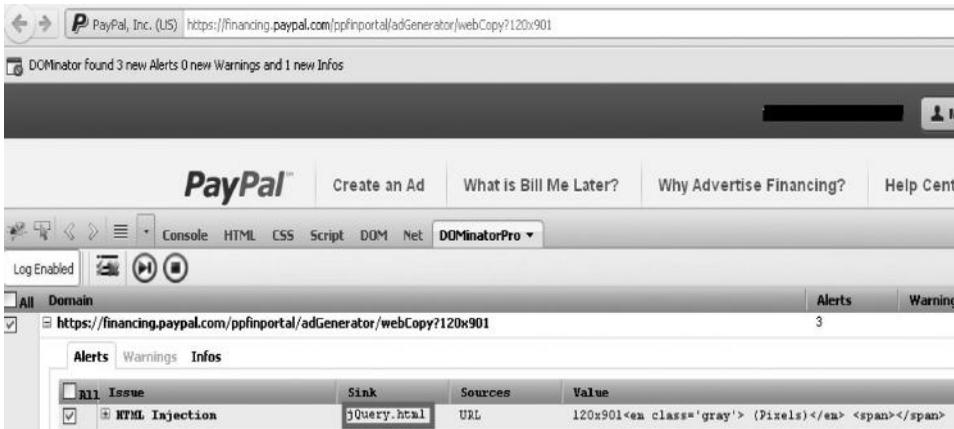
To take a look at how the source was treated before it was passed to a vulnerable sink, we looked at the “Source history” tab. The goal with checking the source history is to see if there is any kind of escaping being performed with the input before it’s passed to the sink.
