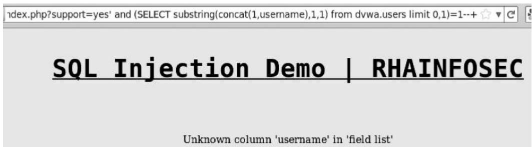
The application returns an error indicating that the column “username” does not exist in the “users” table present in the dvwa database. Let’s now try injecting a column that is present in the table.
