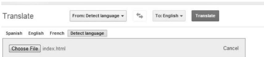
Once you have uploaded the file you want to translate, click on the translate button, and it will try translating the content and display it back to us; since the input is not being sanitized before being reflected to us, it would result in an XSS vulnerability.
