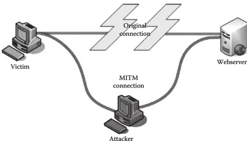
The idea behind a MITM attack is that the attacker places himself in the middle of the communication between a client and a server. Therefore, any communication that is being performed between a client and a server will be captured by the attacker.
