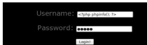
As soon as we visit the logs, the PHP code would be executed, and it would bring us the “phpinfo()” function, which contains a bunch of information about the current php version installed.
