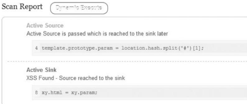
As you can see, the source `location.hash` reaches the sink `div.innerHTML`, which is the root cause of the dom-based XSS.
