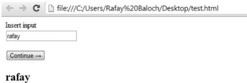
Our input is reflected back to the page; on inspecting it with the Chrome JS console, I found that the input is being inserted into the local storage.
