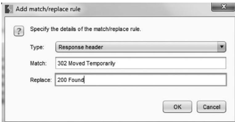
The next time, burp looks at any “302 Moved Temporarily” header, it will replace it with “200 OK” automatically.
