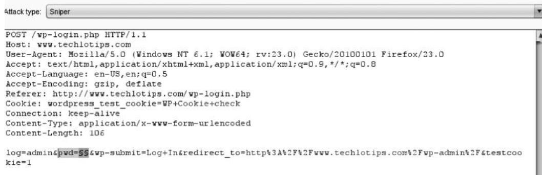
*Step 4*—We will now move to the “payloads” tab, and under payloads options, we will load our wordlist against which we want to test this particular form. For demonstration purpose, I would use the list of top 500 worst passwords by Symantec, for which I will provide the link later.
