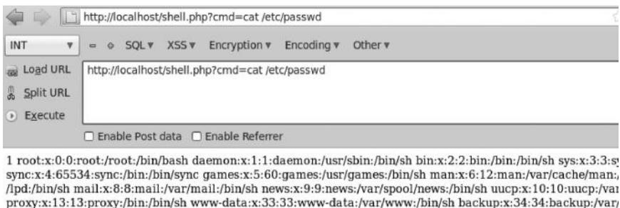
Here, we can execute our commands on the target system, which is Linux based. We would try to read Linux-specific files. If it were running a Windows OS, we would have tried to read files such as “`boot.ini`” or “`winboot.ini`”.
