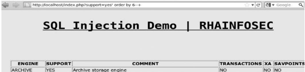
*Note:* The reason we are using ‘ and --± is because our injection type is string. We can figure this out as follows: In a string-based SQL injection, no matter how much you increase the count, you don’t get any results printed on the screen, which means that you need to append a single quote with every query.
