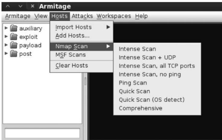
In this case, we choose the first one, which is “intense scan.” Next, a box would prompt asking us to choose targets that we would like to perform the scan against. In this case, I have chosen to scan the whole network, that is, 172.16.222.1–255.
