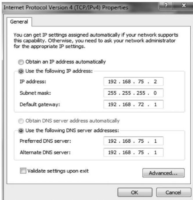
Since our attacker machine is a “BackTrack 5” machine, we would be only interested in making its IP static. We can do it by accessing the WICD manager. We can access it by going to Application → Internet → WICD Network Manager.
