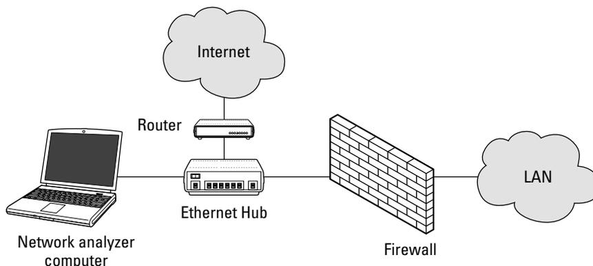
**Figure 9-9:** Connecting a network analyzer outside the firewall.
