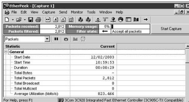
Figure 9-11 shows the Smurf DoS attack on EtherPeek's conversation monitor. Three million bytes were transmitted in this short period of time — from one host.
