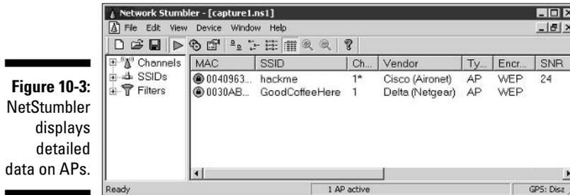
**Figure 10-3:** NetStumbler displays detailed data on APs.
