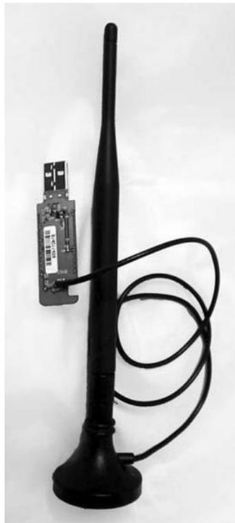
**Figure 8.7** Bluetooth adapter with hacked connector and antenna.
