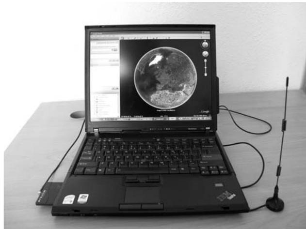
**Figure 7.3** Laptop with omni-directional antenna.
