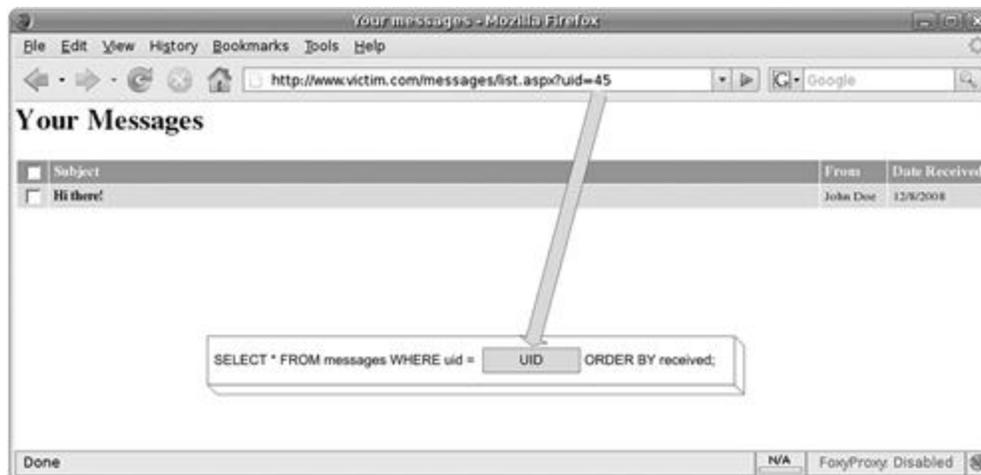
**Figure 2.12** Visual Representation of a Numeric Injection
