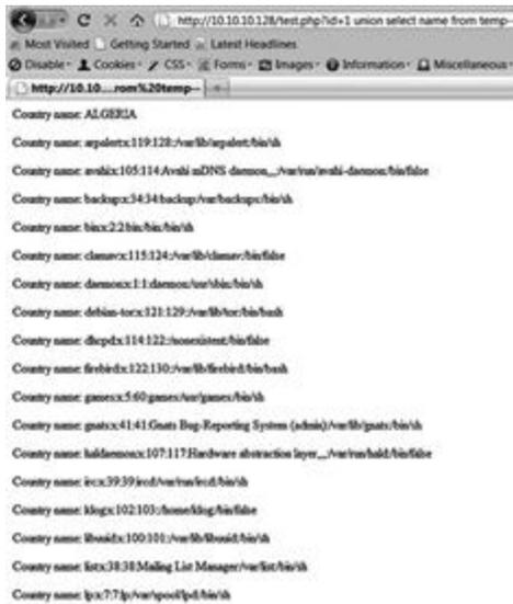
**Figure 6.16** Reading the `/etc/passwd` File on the Database Host
