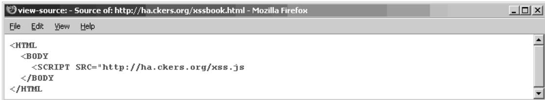
**Figure 3.35** Firefox Generated View-source
