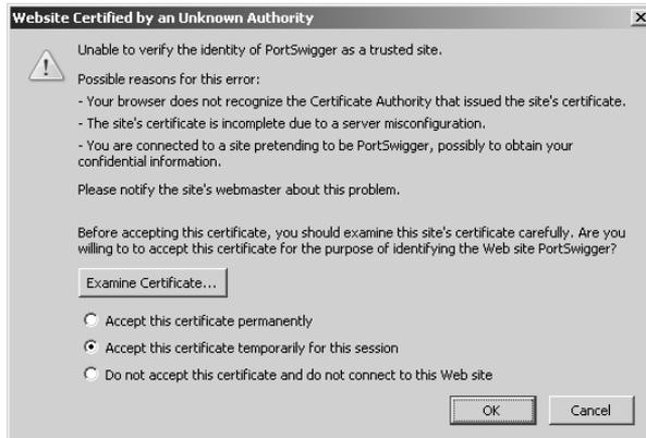
**Figure 19-4:** Using an intercepting proxy with HTTPS communications generates a warning within the attacker's browser.
