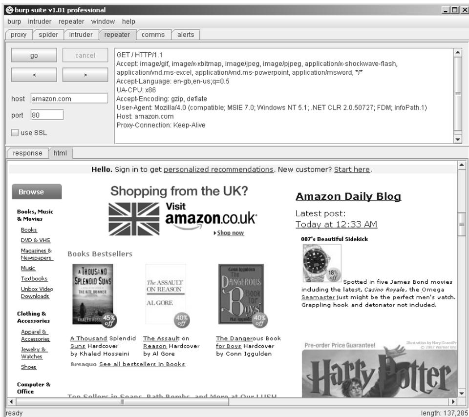
**Figure 19-10:** A request being manually reissued using Burp Repeater
