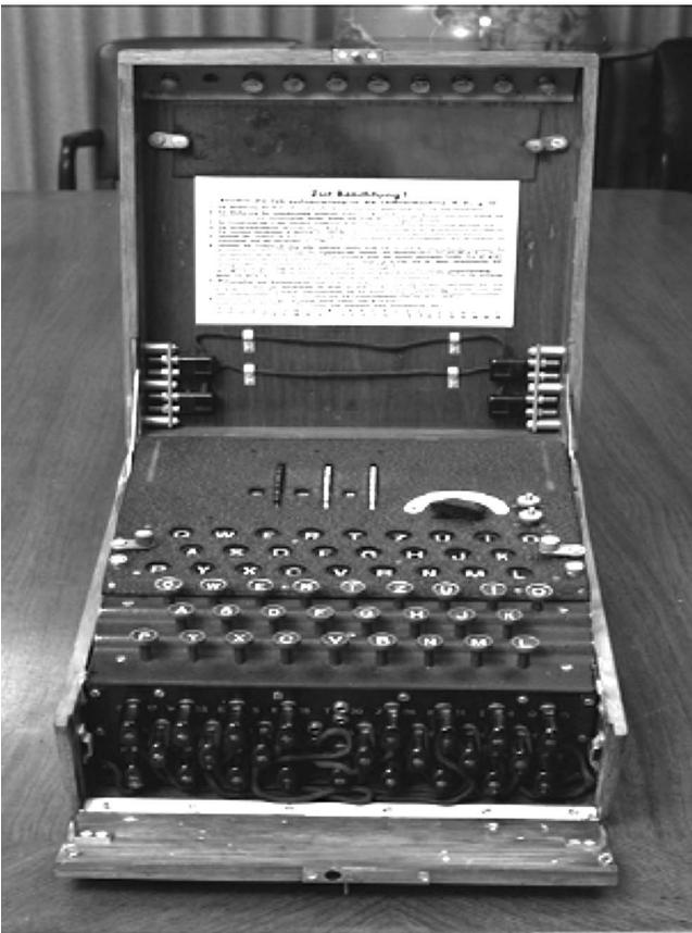
**Figure 6.6** The Enigma machine (Courtesy of NSA).
