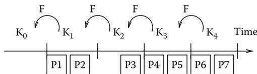
**Figure 14.3** Using a time-released key chain for source authentication. (From Y. Wang, G. Attebury, and B. Ramamurthy, *IEEE Communications Surveys and Tutorials*, Vol. 8, no. 2, pp. 2–23, 2006. With permission.)
