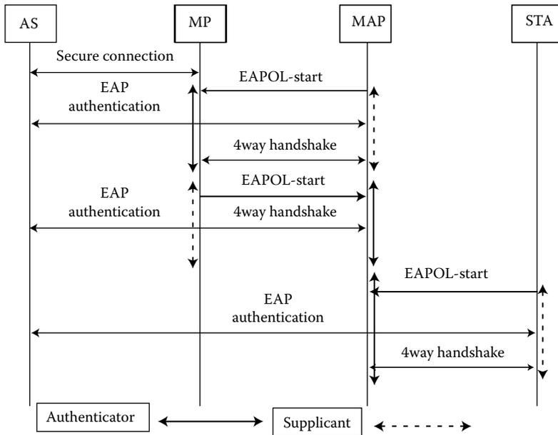
Figure 12.2 Example security exchanges in WLAN mesh.
