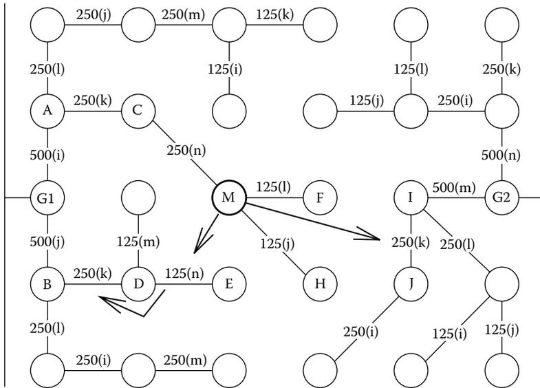
**Figure 3.7** Example WMN with routers physically arranged in grid topology. G1 and G2 are gateways connected to wired network. Edges show routing topology and labels along edges are bandwidth in kbps (channel). For simplicity,  $(k + 1)$ -hop neighbors include immediate physical neighbors only. Arrows show propagation of ripple effect attack from compromised node M.
