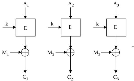
**Figure 11.9** CCM\* encryption block cipher mode.
