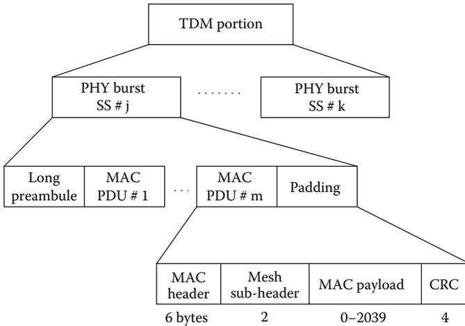
**Figure 2.14** 802.16 data sub-frame in mesh mode.
