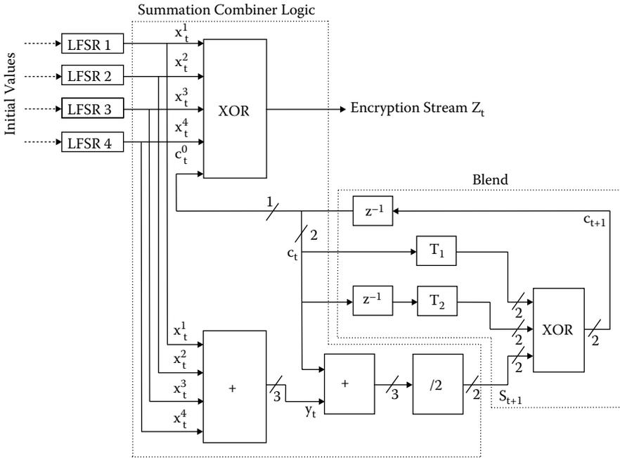
**Figure 11.1** Schematics of the  $E_0$  encryption engine.
