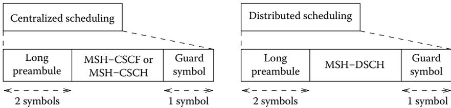
**Figure 2.16** The schedule control sub-frame in mesh mode.
