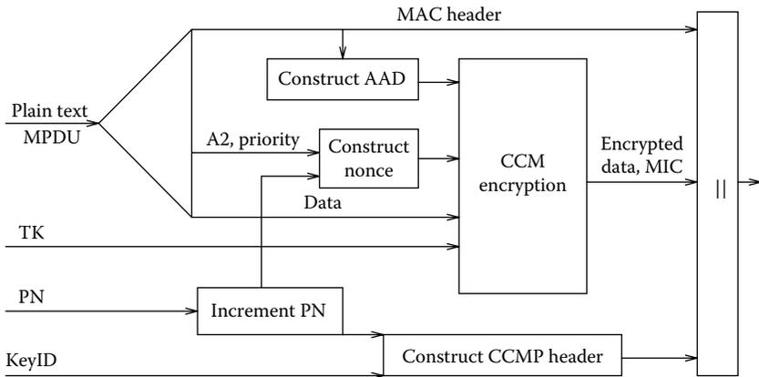
**Figure 3.11** CCMP encryption process and encrypted frame generation [30].
