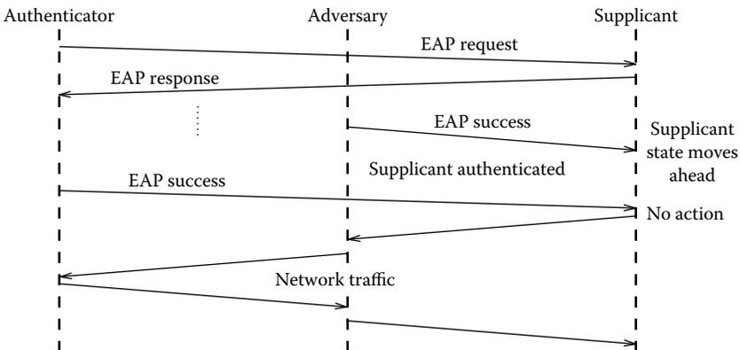
**Figure 3.13** Man-in-the-middle attack on 802.1X authentication mechanism.
