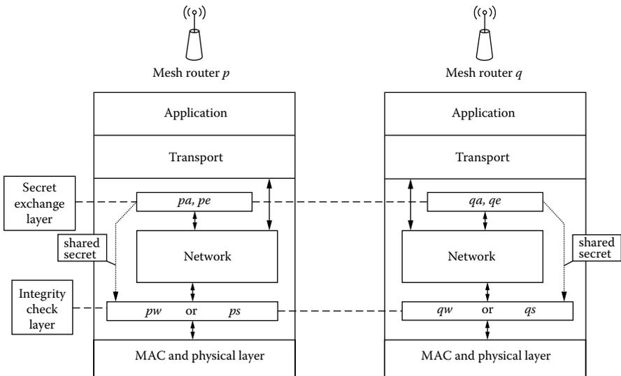
Figure 6.1 Protocol stack for hop integrity protocols.
