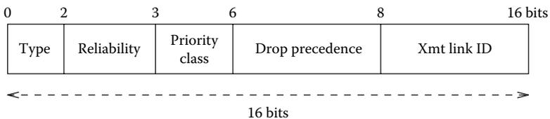
**Figure 2.18** The CID field of a unicast packet.
