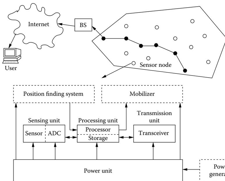
**Figure 14.1** The components of a sensor node. (From Y. Wang, G. Attebury, and B. Ramamurthy, *IEEE Communications Surveys and Tutorials*, Vol. 8, no. 2, pp. 2–23, 2006. With permission.)
