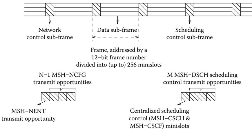
**Figure 2.15** The MAC control sub-frame in mesh mode.
