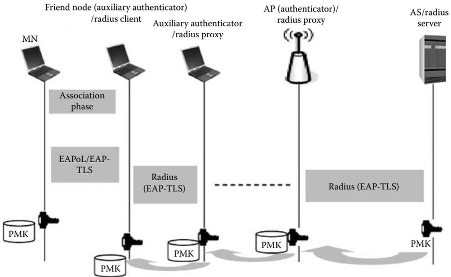
**Figure 8.3** Adapted 802.11i with EAP-TLS for multi-hop communication.
