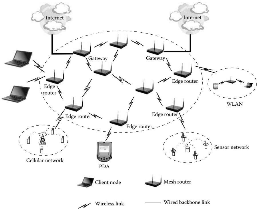
**Figure 1.1** Architecture of a wireless mesh network.
